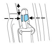
**WARNING:** Position the safety belt height adjusters so that the belt rests across the middle of your shoulder. Failure to adjust the safety belt properly could reduce the effectiveness of the safety belt and increase the risk of injury in a collision.
